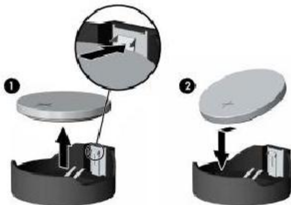
Figure 5-11 Removing the battery from a type 2 holder
