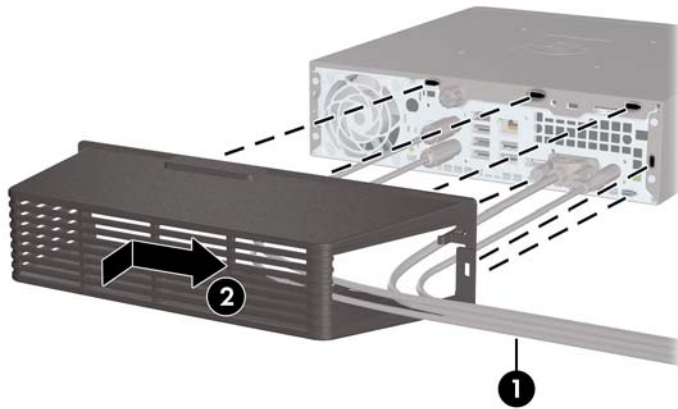
Figure 2-21 Installing a Port Cover
