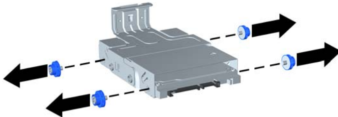
Figure 2-16 Removing the Guide Screws
