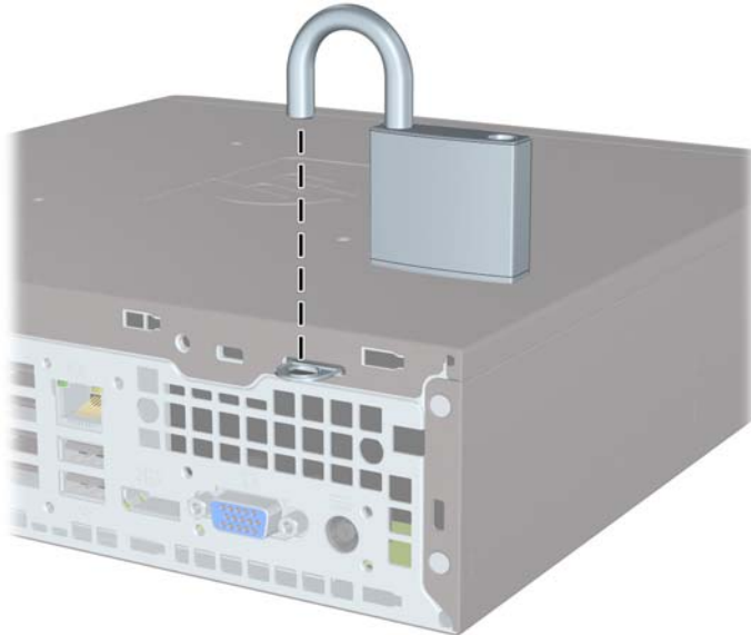
Figure C-3 Installing a Padlock
