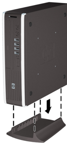
Figure 2-7 Placing the Computer on the Stand
