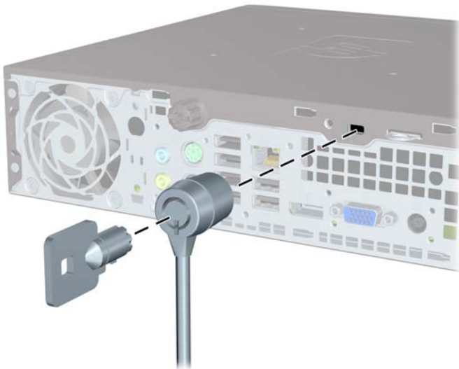
Figure C-1 Installing a Cable Lock with No Port Cover
