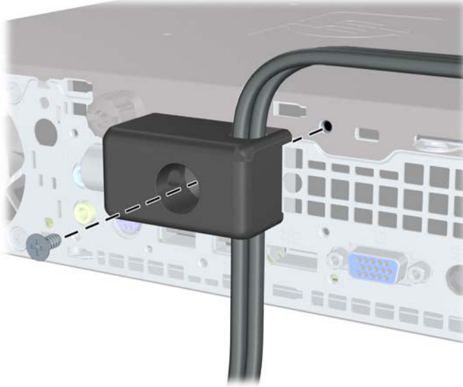
Figure C-6 Attaching the Lock to the Chassis
