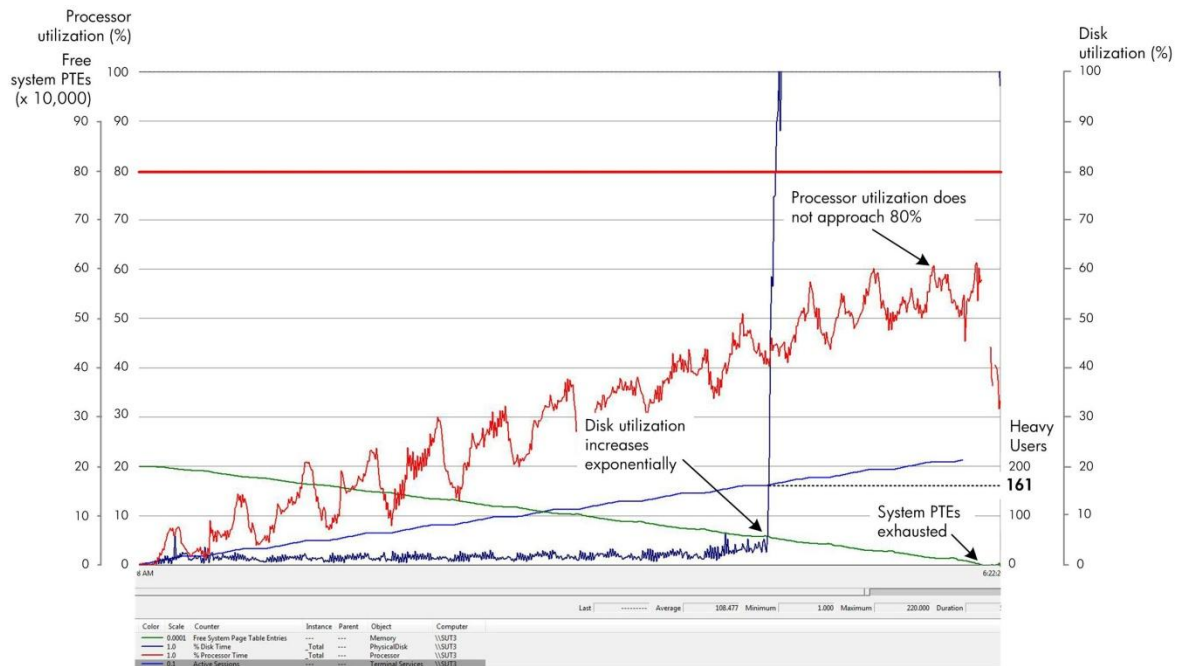
Figure 12. % Processor Time values – showing that 161 Heavy Users were supported when disk utilization began to increase exponentially
