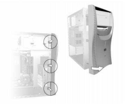
**3** Lay the front panel on a flat surface beside the PC.
