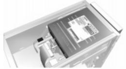
**5** Remove the four retaining screws, then slide the old drive out of the front of the PC.
