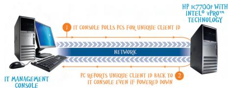
HP Compaq dc7700p desktops equipped with Intel vPro Technology rely on a secure, hardware-based, out-of-band (OOB) communications channel that is always available, enabling third-party software to poll systems for information even if a PC is powered off, its OS is down or its management agents are missing.
