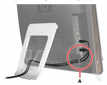
3 Replace the connector cover by aligning the hooks on the right edge of the cover with the slots on the computer, and then pressing it until it snaps into place. Then, route the cables through the notch (B) in the computer stand.
