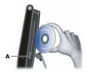
To eject a disc, make sure the power is turned on and then press the eject button (A) on the side of the disc drive. You can also tap the **Windows Vista start button** (5), tap **Computer**, press and hold (or with the mouse, right-click) the CD drive, and then tap **Eject**.
