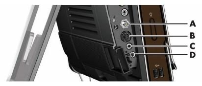
2 If you are using S-Video, connect audio cable from your set-top box to the Audio line in (**C**) connector on the back of the computer. Use with a Y cable to combine RCA left and right channels (white and red).
