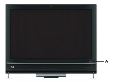
To open the HP TouchSmart software, just press the HP TouchSmart button (A) on the lower-right side of the HP TouchSmart PC.
