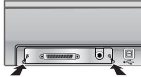
**tighten the two mounting screws**
