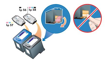
4 Hold the print cartridge with the copper contacts facing the printer, and then slide the print cartridge into the cradle.
