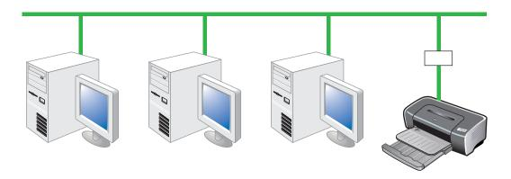
Your printer can be shared in a network environment by connecting it directly to a network via an optional HP Jetdirect external print server. This configuration provides better performance than printing through a computer, flexibility in preparing a location for the printer, and the ability to share the printer with both Windows and Mac OS users.
