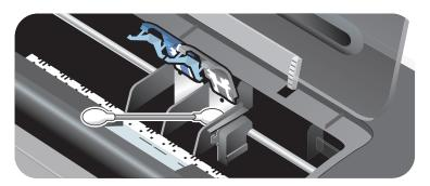
3 Carefully clean the electrical contacts on the print cartridge with a soft, dry, lint-free cloth.
