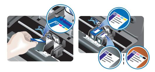
5 Push down on the print cartridge latch until it snaps closed. Make sure the latch does not spring back open.
