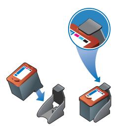
2 To remove the print cartridge from the protector, press down and back on the tab inside the protector to release the print cartridge, and then remove the print cartridge.
