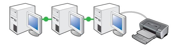
In a locally shared network, the printer is connected directly to the USB or parallel port of a selected computer (known as the server) and is shared by other computers (clients). Use this configuration only in small groups or when usage is low. When many users print to the shared printer, this will slow down the server.
