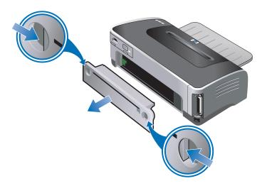
Remove the rear cover from the auto-duplex unit (if installed), remove any paper, and replace the rear cover. If the paper jam is not visible by removing the rear cover, remove the auto-duplex unit to locate the jam.
