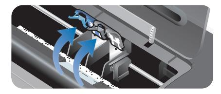
3 If you are replacing a print cartridge, hold the top of the installed print cartridge and slide it out of its cradle. Check the number on the latch against the number on the new print cartridge to make sure you are removing the correct print cartridge.
