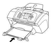
${f 6}$  To prevent paper from possibly falling off the tray, fully extend the output-tray extender.
