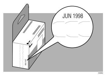
If the print cartridge is in a box, read the "Use Before" date printed on the box.
