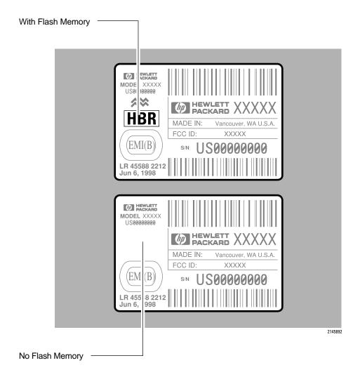
To identify a printer with flash memory, look for the lightning bolt symbol on the serial number label located on the back of the printer. The flash font code found directly below the lightning bolt can be used to identify the language of fonts downloaded into flash memory. Use the following tables to identify the fonts and symbol set(s) loaded into flash memory.
