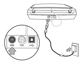
The power supply also has an AC cable that is connected to the power supply on one end and plugged into a power outlet or surge protector on the other end.
