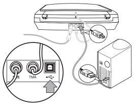
2. Connect the rectangular end of the cable to the computer.
