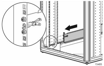
Secure the back end of the rails to the rack.
