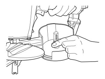
**Step No. 3** – Remove the retainer from a nail coil and place the nail coil in the magazine with the tips of the nails against the loading tray and with about 4 inches of coil unwound.
