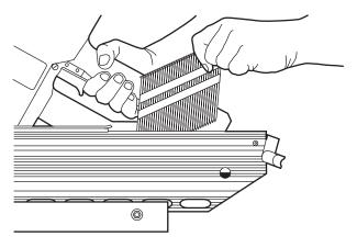
**Step No. 3** – Pivot the follower upward until it releases then slide the follower forward until it contacts the fasteners. The tool is now ready for use.
