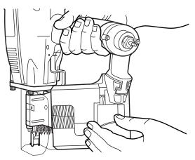
**Step No. 6** - Advance the first nail into driving position by cycling the tool once against a work surface. The nailer is 9 now ready for use.
