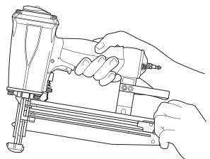
**Step No. 2** – Insert the strip with the point of the fastener facing down towards the bottom of the magazine.
