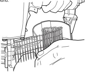
**Step No. 4** - Slide the free strip of nails along the top of the feeder body assembly and place the first nail between the feed claw and the locator.
