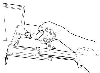
**Step No. 2** – Insert the fastener strip into the magazine rail.
