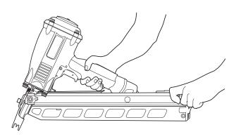
**Step No. 2** – Insert the a strip of fasteners into the top of the magazine with the point of the nails facing the nose area.
