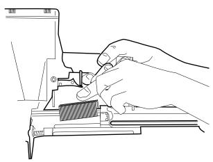
St. . . Io. 3 - Push the magazine firmly towards the front of the tool until it locks in place. The tool is now ready for use.
