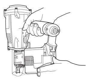
**Step No. 2** – Adjust the loading tray for nail length (if required) by depressing the button on the post and raising or lowering the tray to the desired position.
