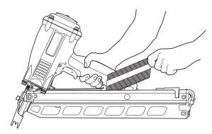
**Step No. 3** – Hold the follower firmly and press the follower latch. Slide the follower forward until it contacts the nails. The tool is now ready for use. NOTE: 5000S models have a follower release button. \_\_\_\_\_
