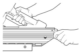
**Step No. 2** – Insert the a strip of fasteners into the top of the magazine with the point of the nails facing the nose area.
