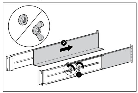
Use the cage nut tool to install cage nuts or clip nuts into the rear of the rack.
