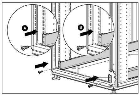
Tighten the wing nuts or hex nuts.
