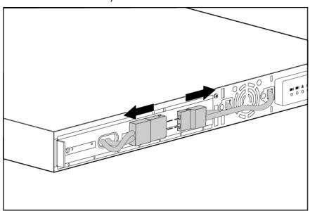
Remove the battery bracket.
