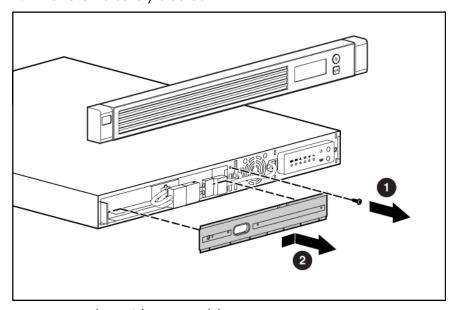
Remove the UPS battery modules.
