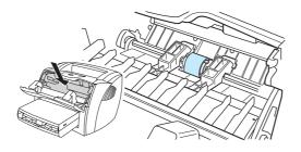
4 Release the small, white tabs on either side of the pickup roller, and rotate the pickup roller toward the front.
