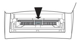
**4** To pry the separation pad up from the spring-loaded base, insert a flat-edged screwdriver in the slot under the separation pad and twist until the tabs are free.
