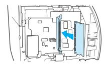
6 Carefully press the DIMM chip into the slot, making sure that it is straight and all the way in (A). The cam latches, located at the top and bottom, should rotate inward. To snap the cam latches into place, press the handles toward each other (B).
