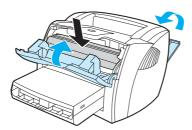
NoteThe pressure release levers automatically close when you close the straight-through output door.After clearing a media jam, you might need to turn the printer off and turn it back on.
