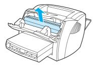
4 With both hands, grasp the side of the media that is most visible (this includes the middle), and carefully pull it free from the printer.
