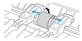
5 Gently pull the pickup roller up and out.
