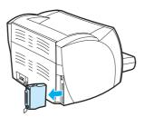
**3** Open the print cartridge door. To open the left side panel, gently pull it out.
