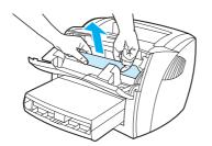
5 If no media is visible, grasp the tab on the right-hand side of the upper media guide and pull it forward. Carefully pull the media up and out of the printer.
