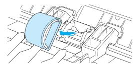
6 Position the new or cleaned part in the slot of the previous pickup roller. See <u>Cleaning the</u> <u>pickup roller</u> for instructions.
