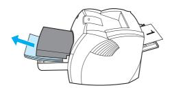
7 Gather the printed pages, turn the printed side down, and straighten the stack before placing it back in the input tray. Side one should be facing down with the bottom edge feeding into the printer first.
