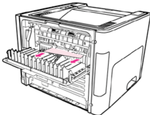
Figure 18: Remove jammed media
