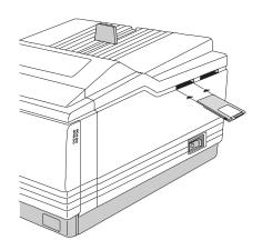
3 Depending on the type of card you are installing, either turn on the printer again or press the Online/Offline key to put the printer back on line.
