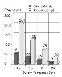
The number of gray levels that your printer can produce depends on the screen frequency and the print resolution. The default value for screen frequency using 600 dpi is 71 lpi. This typically allows 73 different levels of gray. The default value for screen frequency using 300 dpi is 53 lpi. This typically allows 33 different levels of gray. You can change screen frequency through your application or by using the PostScript **setscreen** operator.
