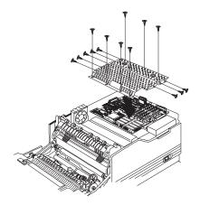
2 Hold the printer's plastic cover over the top of the printer and slide the connector cable back into the printer's connector.
