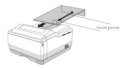
▲ Caution: When removing the paper output ramp, carefully separate the two Velcro pieces so as not to damage the media stopper.
