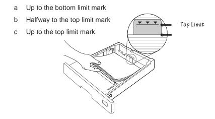
3 Ensure that the paper stack lies flat, does not exceed the top limit mark, and is positioned under the retaining clips.
