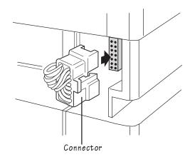
10 Replace the connector cover on the printer.
