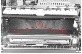
b). From the right side of the printer, remove the pickup clutch alignment guide (callouts 7 & 8). Unplug and free the clutch
