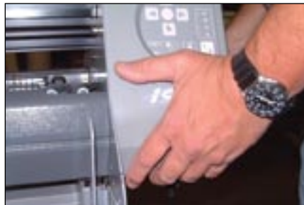
Figure 1. Hold the bottom surfaces of the end covers to avoid injury to your fingers.
