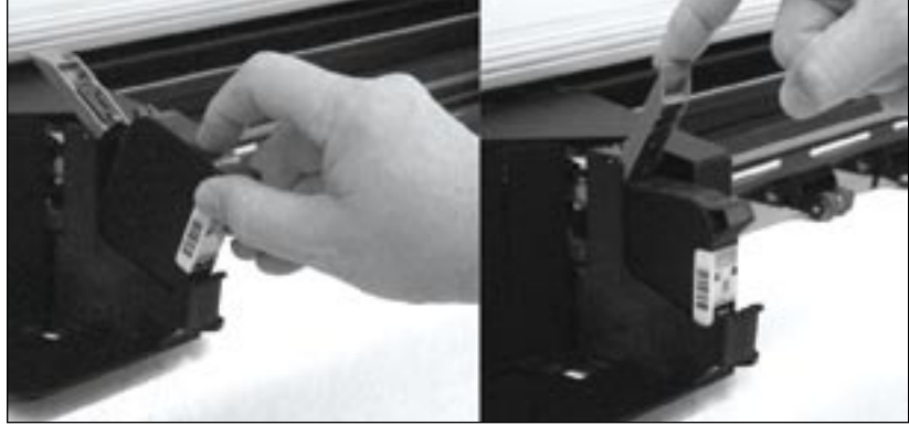
Figure 17. Insert ink cartridge at an angle into the cartridge bay. Lock in place with the stall latch.
