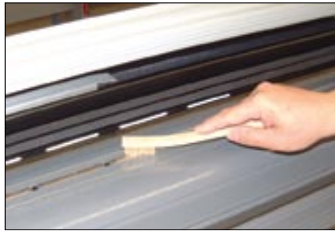
Figure 27. Cleaning the Drive Shaft.
