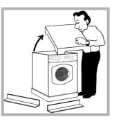
4. Carefully lay the left side of the machine down onto the top cap.
