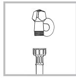
1. Connect the supply pipe by screwing it to a cold water tap using a 3/4 gas threaded connection (see figure). Before performing the connection, allow the water to run freely until it is perfectly clear.
