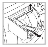
Remove the dispenser by raising it and pulling it out (see figure). Wash it under running
