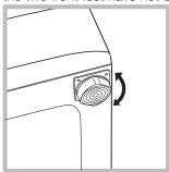
1. Install the washing machine on a flat sturdy floor, without resting it up against walls, cabinets or anything else. 2. If the floor is not perfectly level, compensate for any unevenness by tightening or loosening the adjustable front feet (see figure); the angle of inclination, measured according to the worktop, must not exceed 2°.
