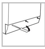
1. using a screwdriver, remove the cover panel on the lower front part of the washing machine (see figure);
