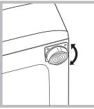
1. Install the washing machine on a flat sturdy floor, without resting it up against walls, cabinets or anything else. 2. If the floor is not perfectly level, compensate for any unevenness by tightening or loosening the adjustable front feet *(see figure);* the angle of inclination, measured according to the worktop, must not exceed 2°.
