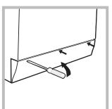
3. using a screwdriver, remove the cover panel on the lower front part of the washing machine (*see figure*).
