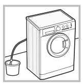
1. remove the plug from the electrical socket. 2. make sure the water level inside the machine is lower than the door opening; if it is not, remove excess water using the drain hose, collecting it in a bucket as indicated in the *figure*.
