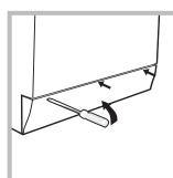
To access the prechamber: 1. using a screwdriver, remove the cover panel on the lower front part of the washing machine (see figure);
