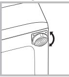
Your machine may make a considerable amount of noise if the two front feet have not been adjusted correctly. 1. Install the washing machine on a flat sturdy floor, without resting it up against walls, cabinets or anything else. 2. If the floor is not perfectly level, compensate for any unevenness by tightening or loosening the adjustable front feet (see figure); the angle of inclination, measured according to the worktop, must not exceed 2°.
