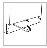
3. using a screwdriver, remove the cover panel on the lower front part of the washing machine (see figure).
