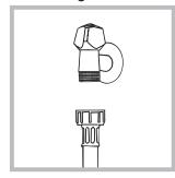
1. Connect the supply pipe by screwing it to a cold water tap using a 3/4 gas threaded connection (see figure). Before performing the connection, allow the water to run freely until it is
