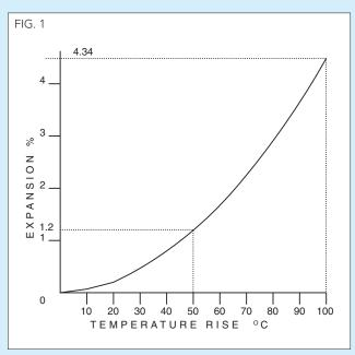
With unvented systems, there are no cistern tanks or open outlets to accommodate expansion. All systems above 15 litre, and some systems of 15 litre or less, employ an expansion vessel or an internal air-gap to accommodate expansion.
