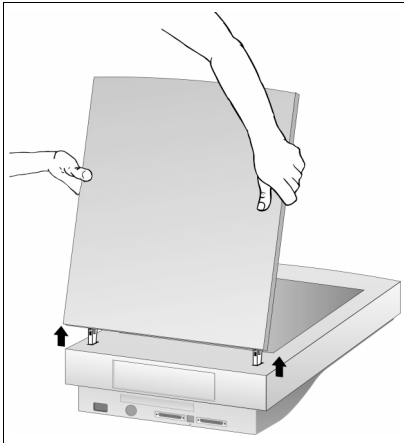
Removing the scanner cover
