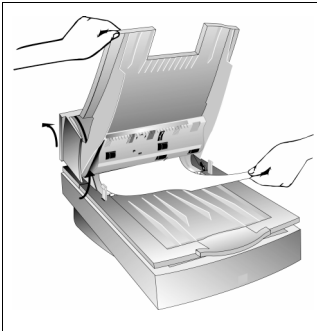
Lifting the input tray to clear the jam
