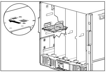
**4.** Push the device bay shelf back until it stops, lift the right side slightly to disengage the two tabs from the divider wall, then rotate the right edge downward (clockwise).
