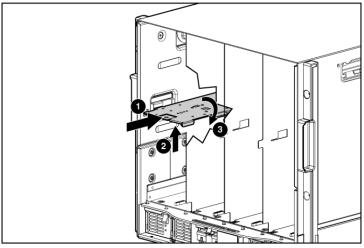
**5.** Lift the left side of the device bay shelf to disengage the three tabs from the divider wall, and then remove it from the enclosure.
