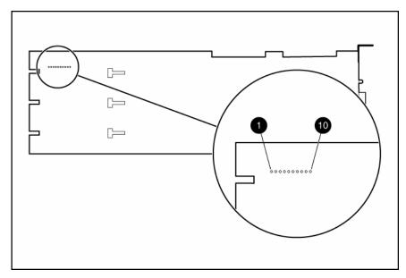
Immediately after the server is powered up, the controller runtime LEDs illuminate briefly in a predetermined pattern as part of the POST sequence. At all other times during server operation, the illumination pattern of the runtime LEDs indicates the status of the controller, as described in the following table.
