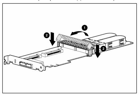
Reinstall the controller in the server.
