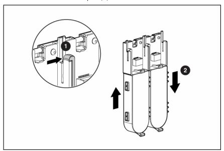
Dispose of the exhausted or faulty battery using environmentally approved procedures ("Battery replacement notice" on page 39).
