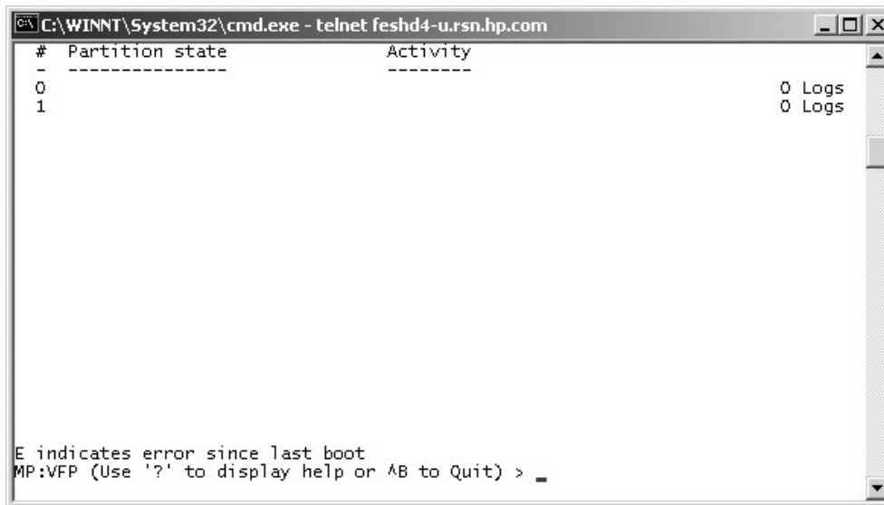
Figure 3-45 Example of Partition State—Cabinet Not Powered Up
