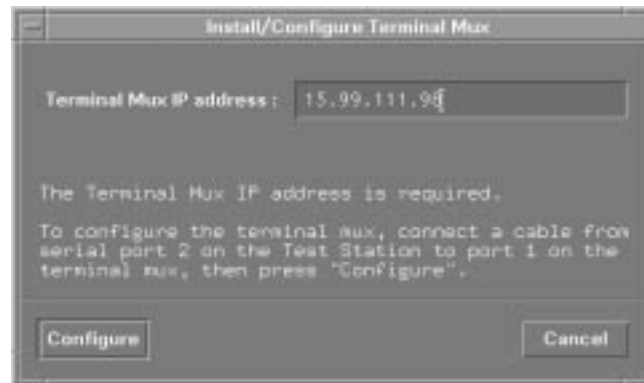
Figure 22 Terminal mux IP address entered into panel
