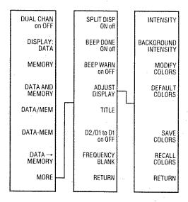
INTENSITY Sets the CRT intensity as a percentage of the brightest setting. The factory-set default value is stored in non-volatile memory.
