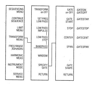
GATE Turns the gate on and off. Although the gate is set in the time domain, it is actually applied to the frequency domain data.
