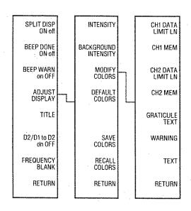
Note: these keys (except return) lead to a second color menu that allows modification of tint, brightness, and color. If varying tint has no visible effect, increase the color percentage first.
