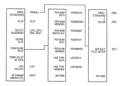
[STANDARD] Copies the HP 8753 display onto an external printer. Identifies the printer selected; [STANDARD] (for black and white), or [COLOR]. The HP 8753 must be in either system controller or pass control mode.
