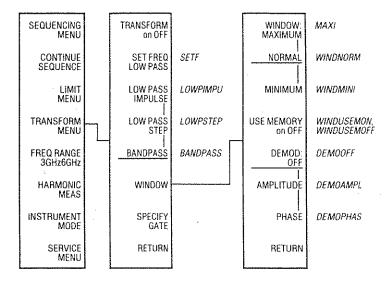
**TRANSFORM** on OFF Turns on the transform and displays the time domain response of a linear frequency sweep, or the frequency domain response of a CW time sweep.
