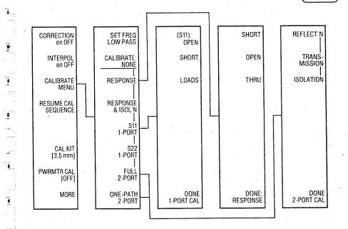
SET FREQ LOW PASS Changes the frequency sweep to accommodate time domain low pass mode (option 010). If this mode is used, the frequencies must be set before calibration.
