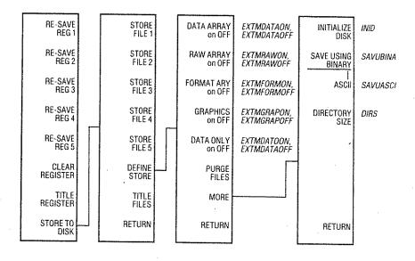
The disk access functions are controlled through the [STORE TO DISK] and [LOAD FROM DISK] menus under the [SAVE] and [RECALL] keys, respectively. In addition to the complete instrument state, some information that is not included in the internal registers can be stored on disk.
