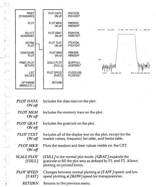
**PLOT DATA** Includes the data trace on the plot. ON off
