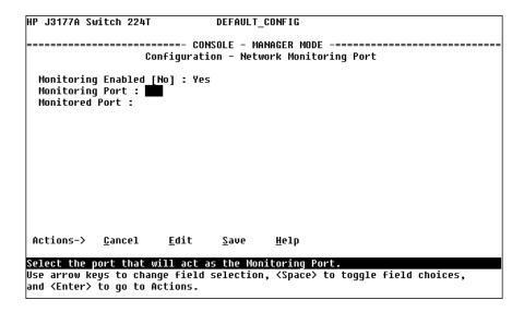
Figure 4-14. Example of Selecting a Monitoring Port
