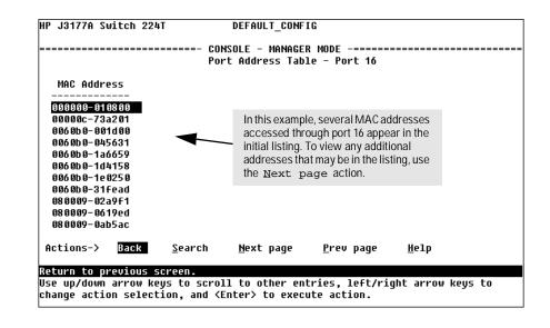
Figure 5-8. Example of a Port Address Table for a Specific Port
