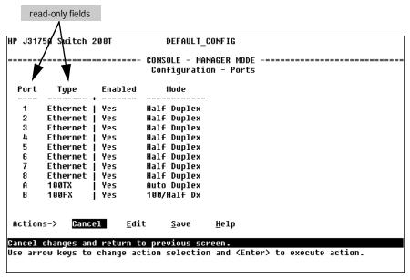
Figure 4-4. Example of the Port Configuration Screen
