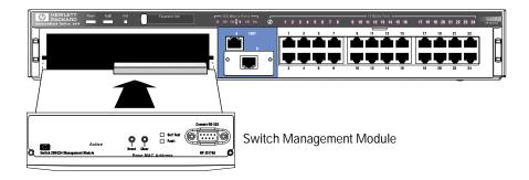
Figure 1-1. The Switch 208/224 Management Module
