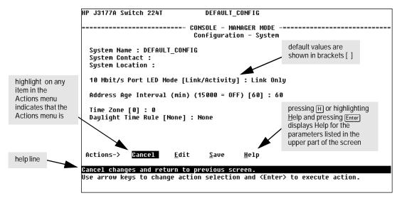
Figure 4-1. Example Showing How To Display Help
