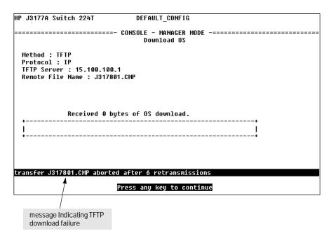
Figure C-3. Example of Message for Download Failure
