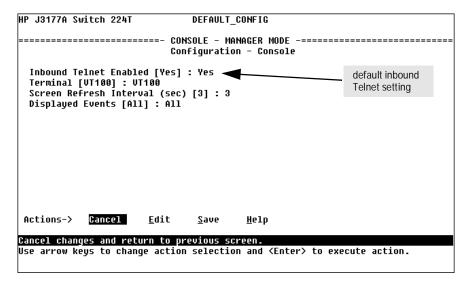
Figure 4-11. The Console Configuration Screen (Default Values)
