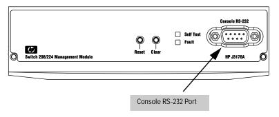
Figure 3-1. Connecting a PC or Terminal to the Console RS-232 Port
