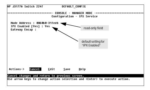
Figure 4-5. The IPX Service Configuration Screen (Default Values)
