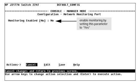
Figure 4-13. The Default Network Monitoring Configuration Screen
