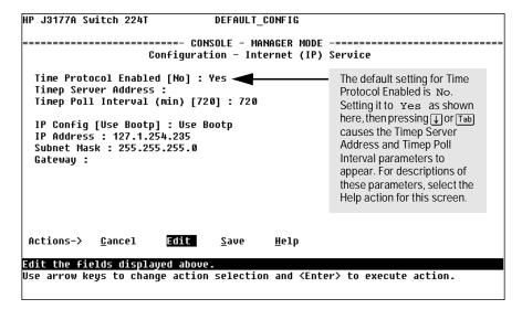
Figure 4-6. Example of the IP Service Configuration Screen (Default Values)
