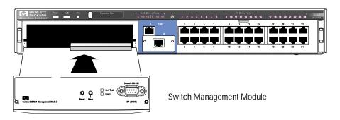
Figure 1-3. Insert the Switch Management Module
