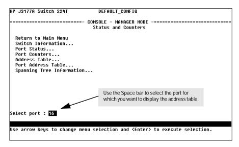
Figure 5-7. Example of How To Access the Port Address Table
