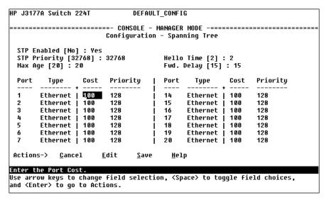
Figure 4-12. Example of the STP Configuration Screen
