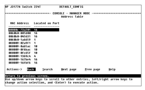
Figure 5-6. Example of the Address Table
