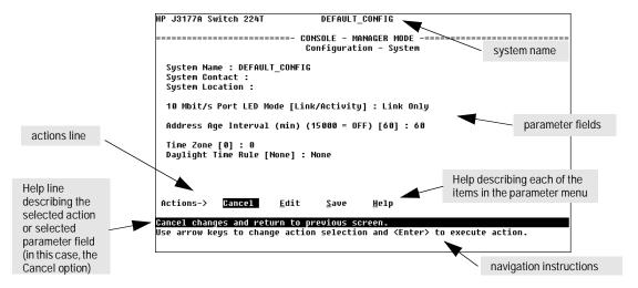
Figure 3-4. Elements of Screen Structure
