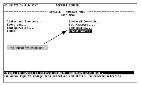
Figure 3-6. The Reboot Switch Option in the Main Menu
