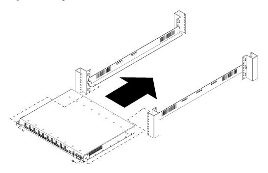
10. Slide the plenum shroud into the front side of the rack. Align the holes in the plenum shroud brackets with the holes in the assembled rails and outer posts.
