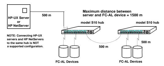
Cascaded hubs must have the same firmware versions to operate properly. If you are using Fibre Channel Manager to manage cascaded hubs, configure the hub that has the LAN (ethernet) connection as a parent hub and the remaining hub as a child hub (see Configuring Cascaded Hubs on page 60).
