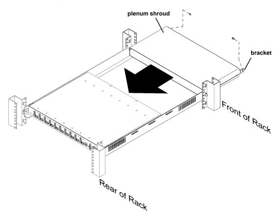
Figure 12 Hub Correctly Installed in a Rack
