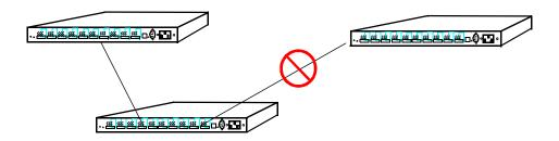
Connecting an HP-UX server and HP NetServer to the same hub is NOT a supported configuration.
