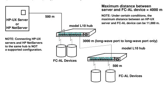
Cascaded hubs must have the same firmware versions to operate properly. If you are using Fibre Channel Manager to manage cascaded hubs, configure the hub that has the LAN (ethernet) connection as a parent hub and the remaining hub as a child hub (see page 60 for more information).
