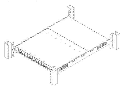
12. Plug the PDU cable into the cabinet PDU when you are ready to power on the hub. The hub finishes the self-test in less than 15 seconds. Verify that the hub passes the self-test.
