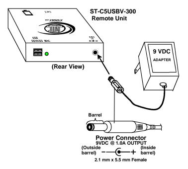
Figure 9- Connect AC adapters
