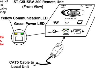
Figure 8- Connect CAT5 cable to the Remote Unit
