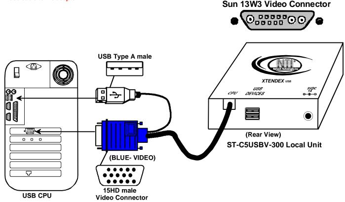
Figure 1- Connect the Local Unit to a CPU
