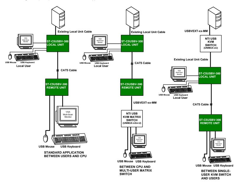
Figure 11- Examples of common applications for the ST-C5USBV-300 USB KVM Extender
