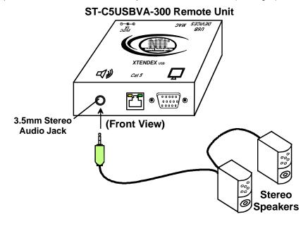
Figure 7- Connect remote self-powered speakers to Remote Unit
