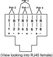
Figure 12- Pin positions in female RJ45 connector
