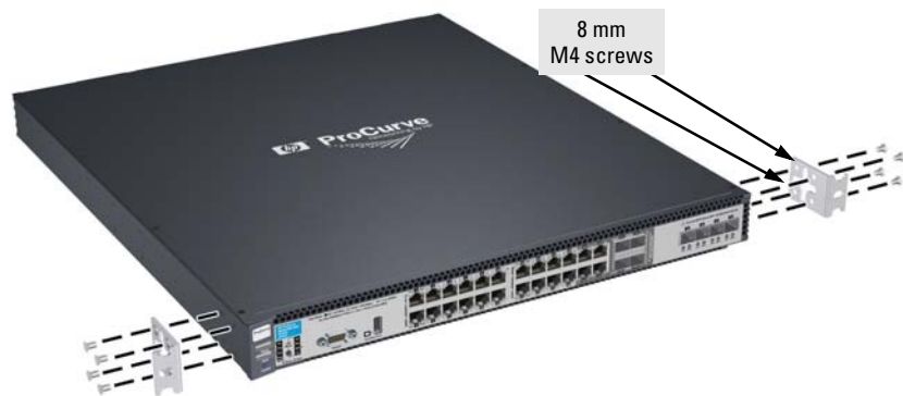
Figure 2-6. Example attaching mounting brackets
