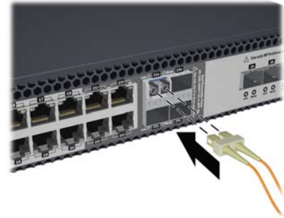
Figure 2-14. Connecting a Fiber cable connector
