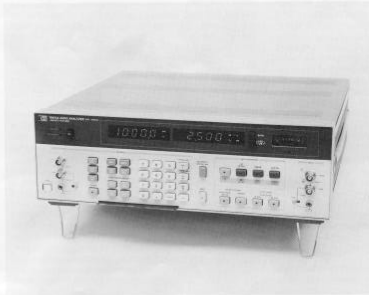
Fig. 1. Model 8903A Audio Analyzer makes the accurate measurements needed to characterize systems and signals in its frequency range of 20 Hz to 100 kHz. It has applications in general audio testing, transceiver testing, and automatic systems. Microprocessor control makes it automatic and easy to use.
