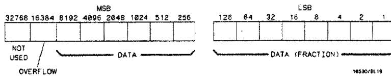
Figure 26-3. Word Data Structure
