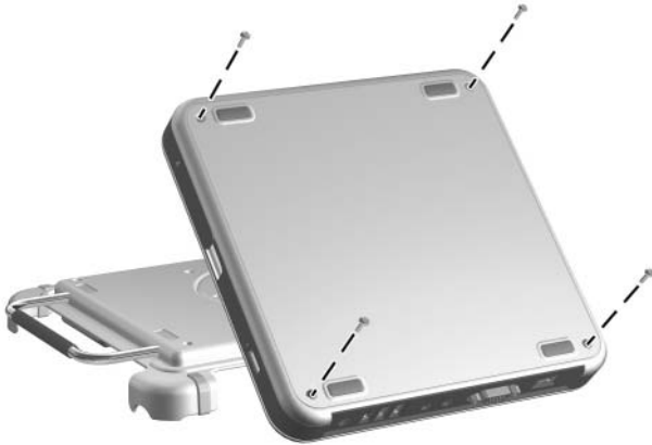
Removing the Top Case Screws
