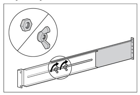
Install the rear stabilization bracket using wing nuts. Wait until the unit is installed and the brackets are adjusted before tightening the nuts.
