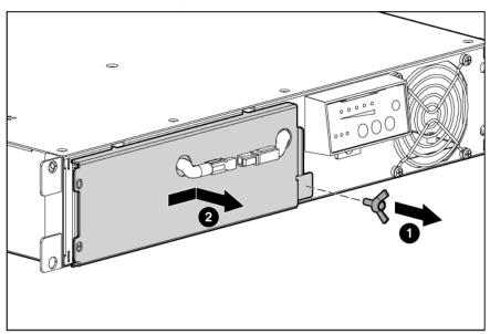
Remove the UPS battery modules.
