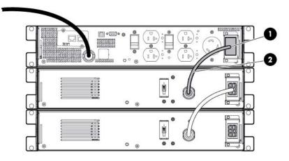
Attach the ERM connector bracket to the UPS as a cord retention bracket for the ERM cable.
