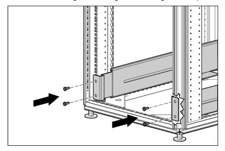
Tighten the wing nuts or hex nuts.
