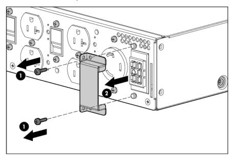
Connect the ERM cable (2) in the socket (1) at the rear of the UPS.
