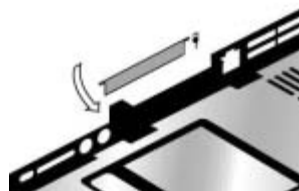
Figure 2-37. Removing a PCMCIA Door
