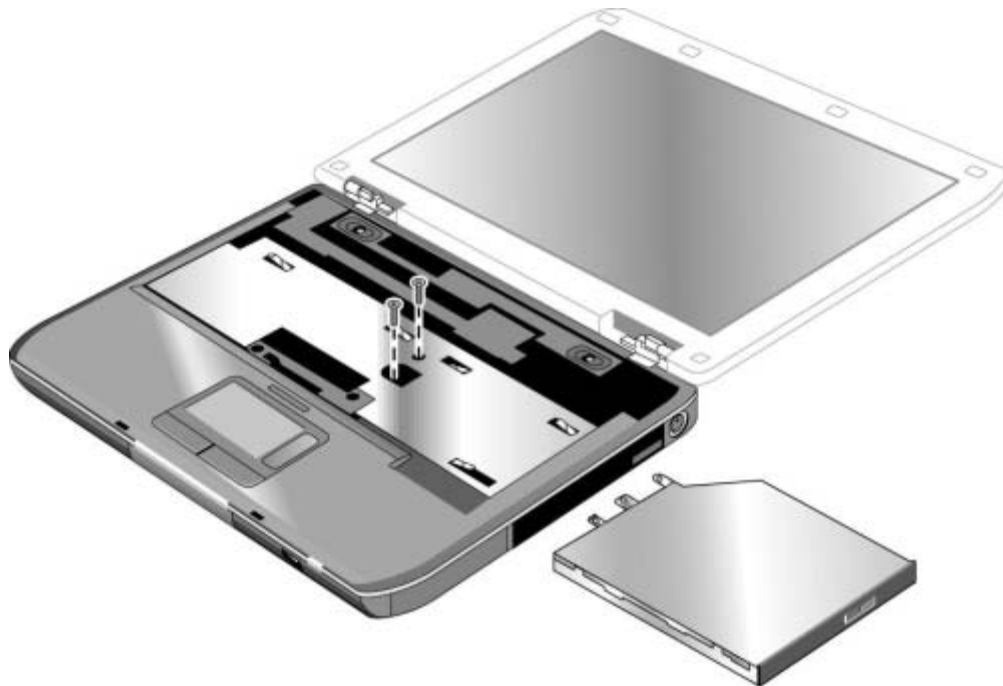
Figure 2-15. Removing the CD/DVD Drive
