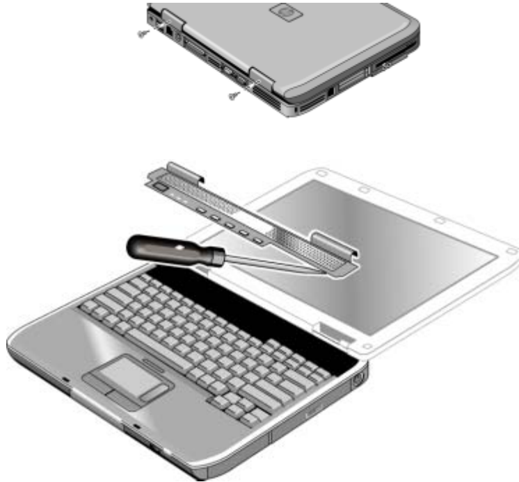
Figure 2-9. Removing the Keyboard Cover
