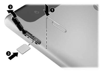
**5**. Insert the SIM into the SIM slot (3), and then push to lock it.
