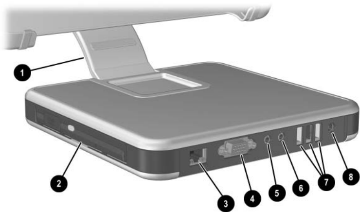
Docking Station Front and Left-Side Components
