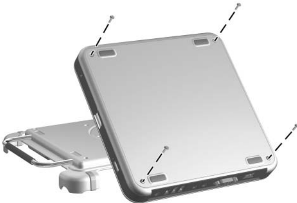
Removing the Top Case Screws
