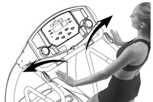
4. Use both sensors to stop belt.
