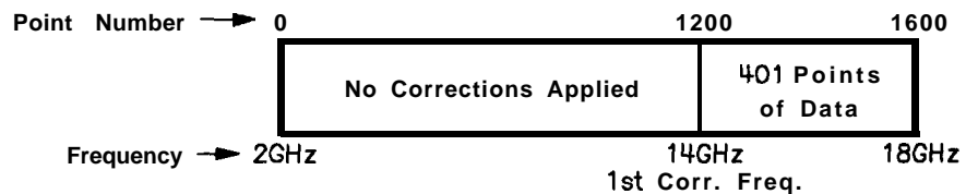
Figure F-4. Array Configuration when the Correction Data Frequency Span is a Subset of the Synthesizer Frequency Span
