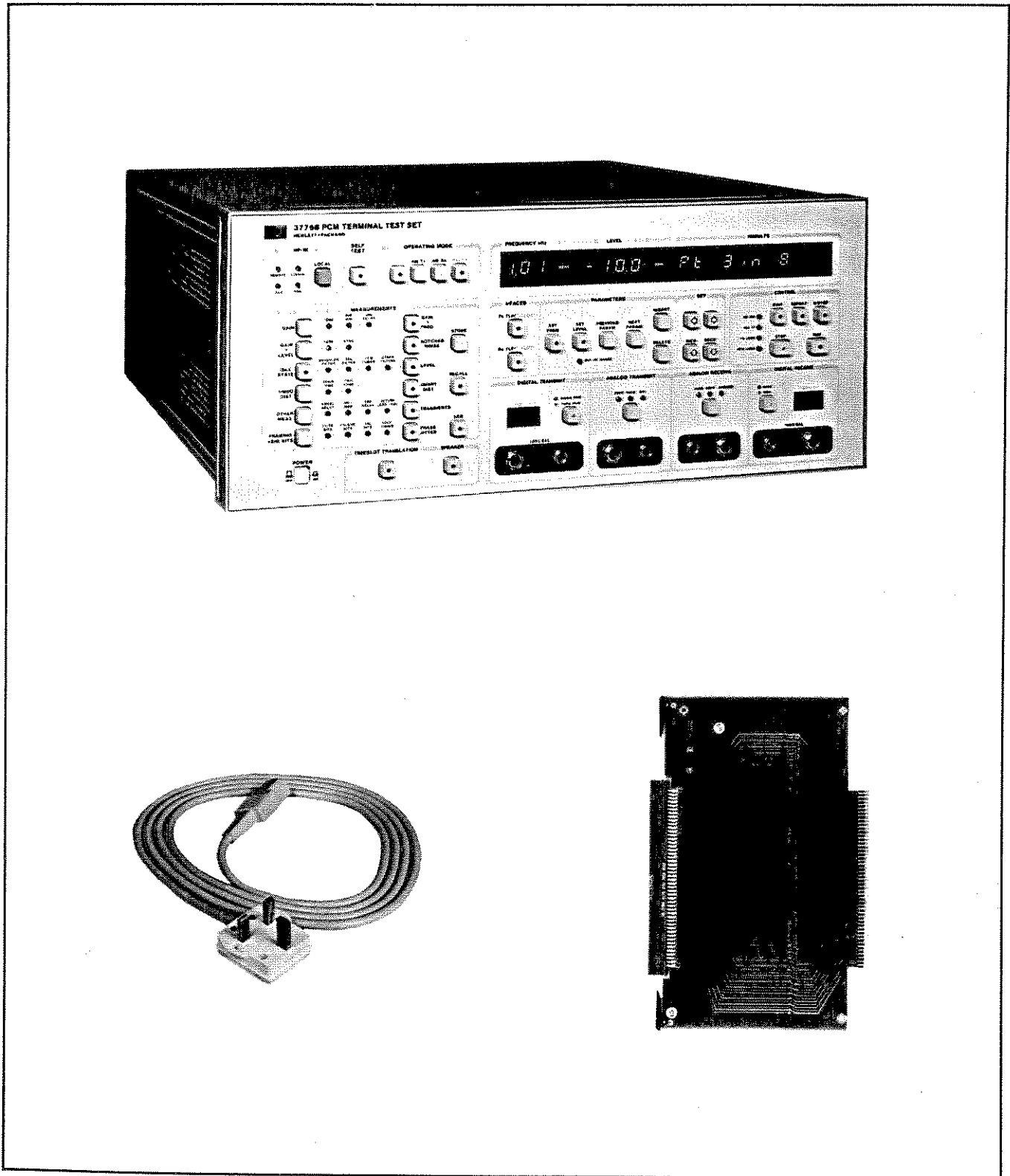
Figure 1-1 The 3776B PCM Terminal Test Set with Accessories supplied
