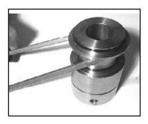
9) Remove seal case (37) from seal sleeve (35).
